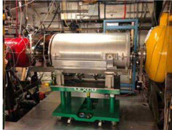
AT-TPC (Active-Target Time Projection Chamber) at the target location of the S800 for the experimental setup (before cabling).
