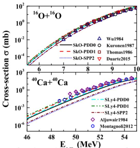
**Figure:** Cross-sections for the sub-barrier fusion of symmetric systems  $^{16}\text{O}+^{16}\text{O}$  and  $^{40}\text{Ca}+^{40}\text{Ca}$  as a function of energy in the center of mass frame ( $E_{cm}$ ) calculated for different DFM potentials and density profiles.
