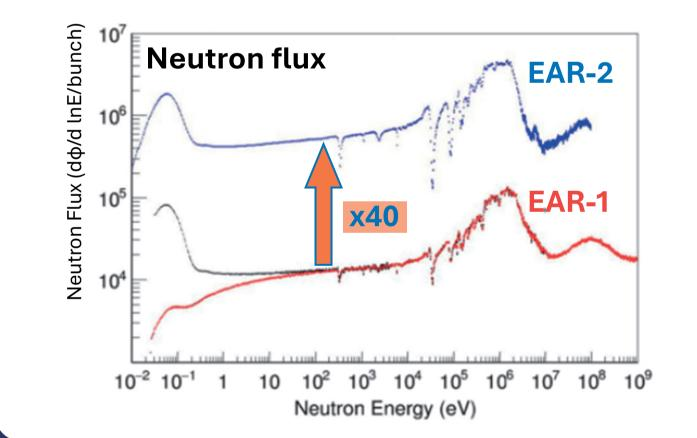
The construction of **EAR-2**, closer to spallation the target and characterized by a higher neutron flux, has enabled the measurement of samples with high radioactivity and/or small mass (down to µg). As a result, the costly <sup>64</sup>Ni could also be studied.
