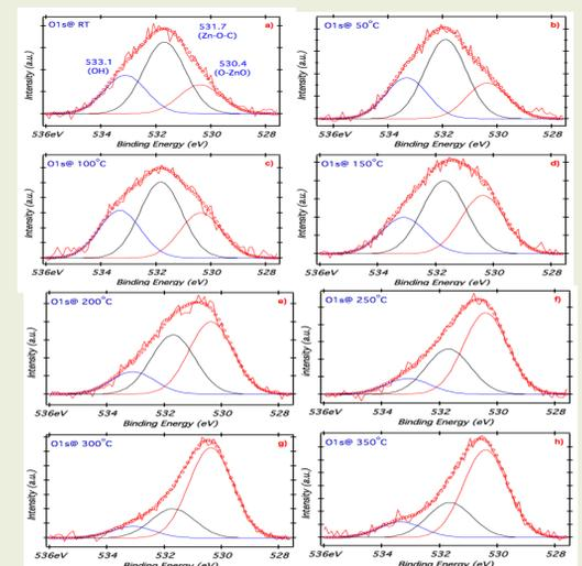
Figure 4 O1s core level photoemission spectra received from as-grown rGO–ZnO core shell hybrid nanostructures at room temperature (RT), and during annealing at 50°C, 100 °C, 150 °C, 200 °C, 250 °C, 300 °C and at 350 °C
