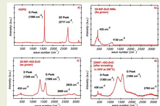
Figure 5, Raman spectra obtained from HOPG (a), as grown pure ZnO NWs on nickel foam substrate (b), as grown rGO – ZnO core shell nanowire hybrid structures on 3D nickel foam substrate (c), and after annealing rGO – ZnO core shell nanowire hybrid structures at 350°C (After performing XPS studies)
