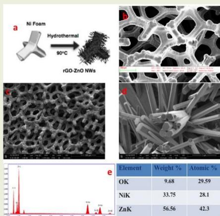
Figure 1 (a) Schematic illustration of growth of ZnO nanostructures and rGO–ZnO hybrid nanostructures by hydrothermal process in a single step process. SEM images, (b) collected from bare nickel foam substrate, (c) micrograph of Ni foam after growth of ZnO NWs nanostructures, (d) High-resolution image of as grown Pure ZnO nanostructures on Nickel foam. (e) EDS spectra received from as grown pure ZnO nanostructures.
