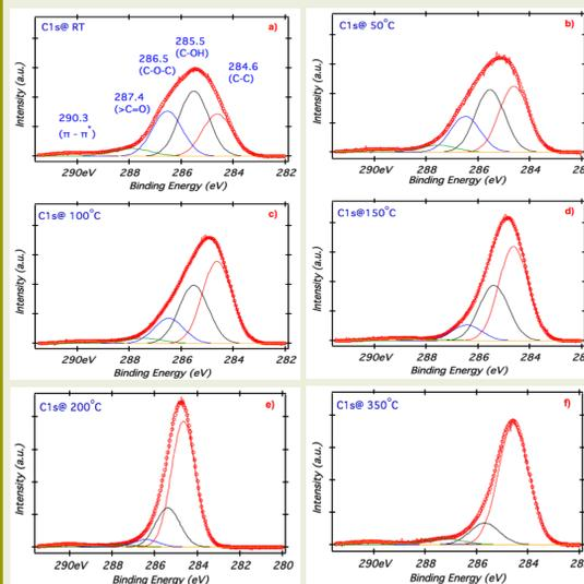
Figure 3 C1s core level spectra collected from as grown rGO–ZnO core shell hybrid nanostructures at RT (25 °C), and during annealing at 50°C, 100 °C, 150 °C, 200 °C, and at 350 °C.
