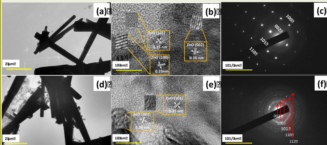
Figure 6 TEM results of as synthesized pristine ZnO nanostructures, (a) & (b) low & high resolution images, respectively and SAED pattern. TEM images of as grown rGO - ZnO (10 wt.%) hybrid nanostructures (d) & (e) low & high resolution images, respectively, and SAED pattern of ZnO-rGO hybrid nanostructures (c).
