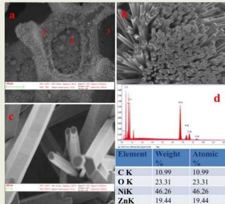
Figure 2, SEM images, (a) Low magnification micrograph of as grown rGO–ZnO hybrid nanostructures on the nickel foam substrate. The numbers 1, 2, 3 in the image refer to branches of the nickel foam at three different depths. (b, c) SEM images of same sample at lower and higher magnifications. (d) EDS spectra collected from as grown rGO–ZnO hybrid nanostructures
