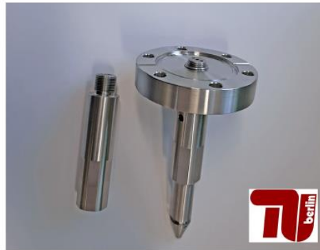
Fig. 5 Elliptical monocalillary and holder for focussing and differential pumping
