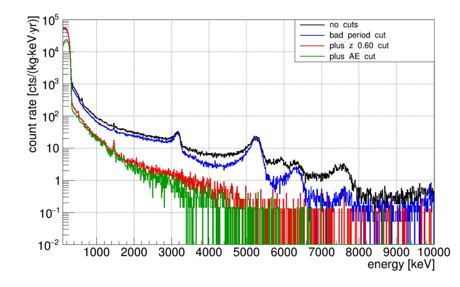
The detector's background is reduced significantly by the application of various cuts:
