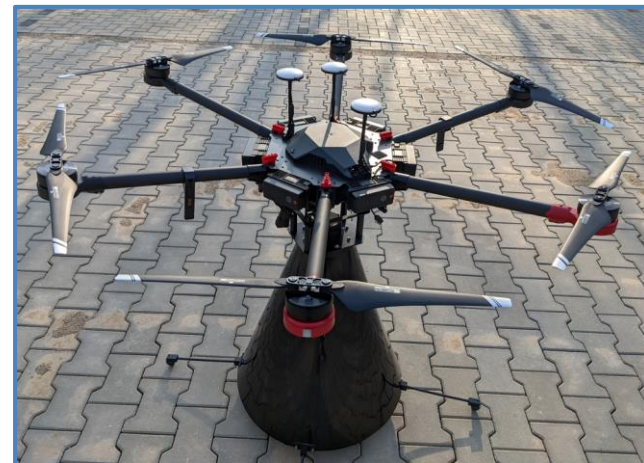
Fresnel-Lense system on a drone to map contamination from a distance
