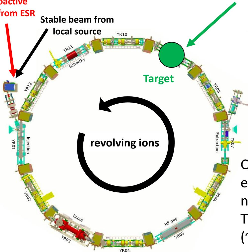
It has one straight section for experiments with an **internal cryogenic microdroplet target**.
