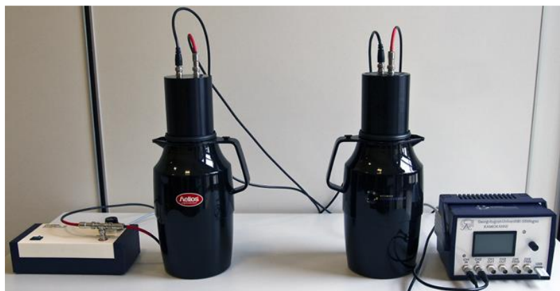
Kamio-Can: Coffee pot used as Cherenkov detector
