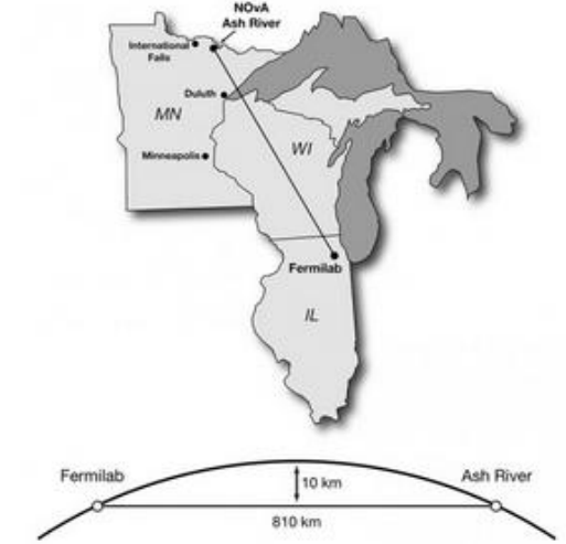
The 500-mile (800 km) subterranean path of the NOvA neutrino beam (Fermilab)
