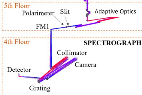
Optical path of the GREGOR telescope and the GRIS spectrograph
