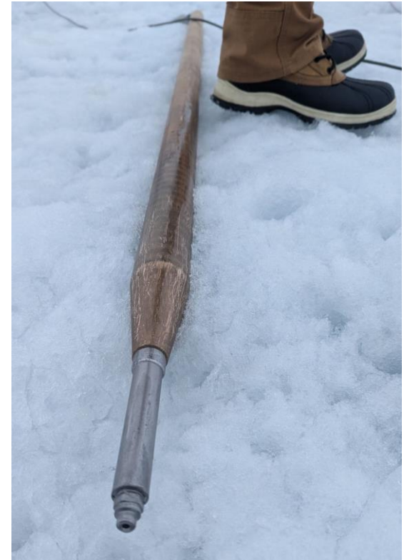
Nozzel stem 2m long , 50mm OD brass pipe (40kg) equipped with high pressure nozzle (Size 040 strait jet)
