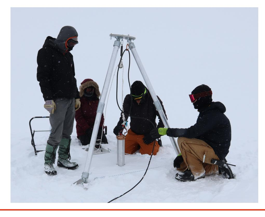
Its successful use by the RNO-G team has demonstrated the feasibility of replacing traditional augering techniques with autonomous melting systems for future deployments.
