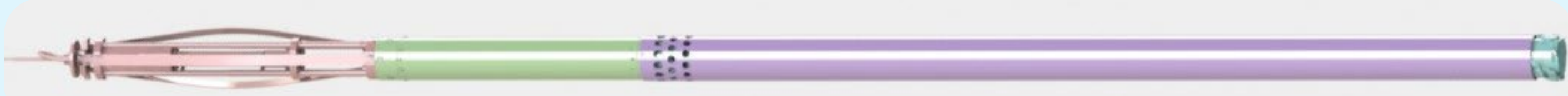
Figure 4. Conceptual image of the Shallow Wet Drill sonde showing the anti-torque section (red), motor section (green), and 1m barrel set (purple).
