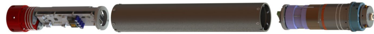
Figure 9. Exploded view of motor section with updated electronics package (left), housing (center), motor and gear box assembly (right).
