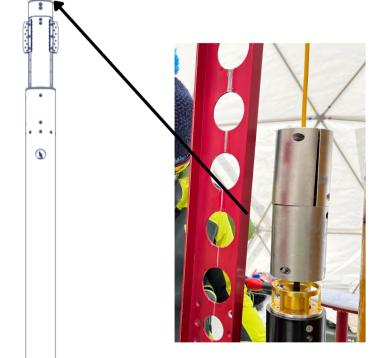
Both the EM100 and ET85 were equipped with additional weights when working underwater. In the picture, each weight module is 5 kg. To extend the cable life, weights removed not were necessary.
