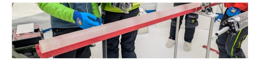
Results with **EM100** (HDF2023 and GC2025) Average recovered core length: 83 ± 20 cm Average recovered core Ø: 101 ± 1 mm Feed rate: **3 - 8 mm s**<sup>-1</sup> Production rate: 6 ± 2 m h<sup>-1</sup>
