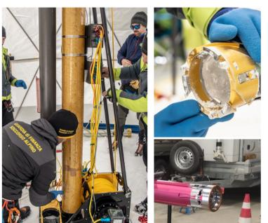
**Electromechanical drill** (**EM100**, HDF2023, GC2025) Core barrel length: 110 cm Core diameter: 100 mm
