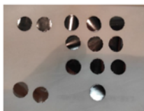
Fig. 6: ^{104}\text{Fe} disks of 10 \mu\text{m} thickness, obtained via cold rolling. (Credit: INFN-LNS)
