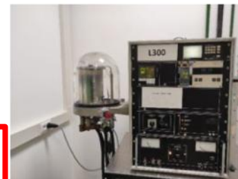
Fig. 10: Leybold L300 evaporator with 2 thermic sources. (Credit: INFN-LNS)
