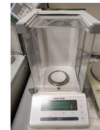
Fig. 12: 5 digits analytical balance. (Credit: INFN-LNS)
