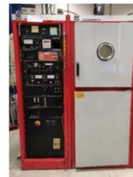
Fig. 11: Leybold L560 evaporator with 1 thermic source and electron beam. (Credit: INFN-LNS)
