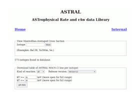
ASTRAL, the ASTrophysical Rate and rAw data Library, collects recommended neutron capture cross sections required for s-process nucleosynthesis calculations. As measured data are typically cross section ratios between the isotope under investigation and a reference cross section, ASTRAL does not only store the cross section but also the raw value, allowing to accommodate updates of the reference cross sections.
