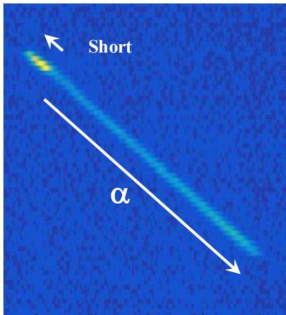
$\alpha$  Track length converted to energy using SRIM
