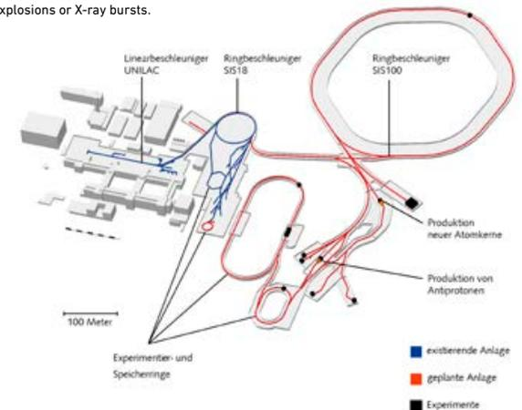
Above: The new Facility for Antiproton and Ion Research (FAIR) at GSI, Darmstadt, Germany. The existing GSI facility is shown on the left, in dark blue the existing GSI accelerator facilities and ion sources. The new FAIR complex is displayed in red.
