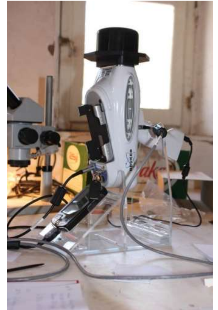
In situ measurement with pXRF of metallurgical relicts in the fragments
