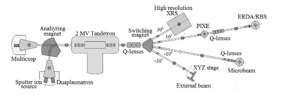
Schematic view of the accelerating system at IJS
