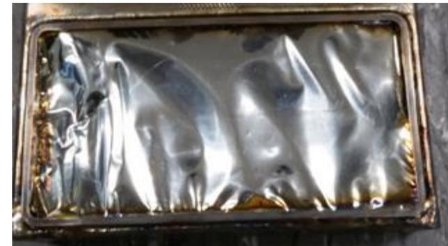
Many failures until finding the appropriate procedure for soldering the window and making it vacuum tight!
