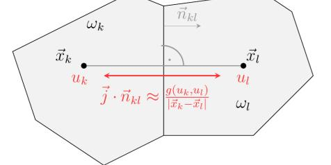
• Solver for coupled convection-reaction-diffusion systems
