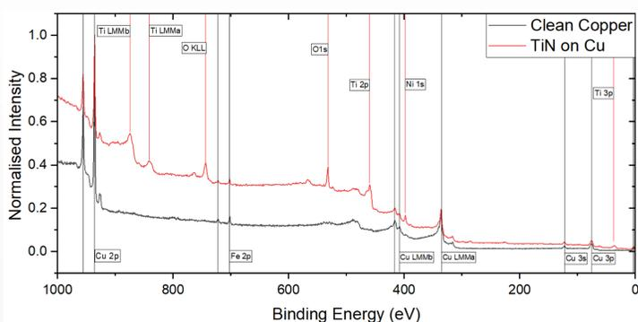
Figure 3: The XPS spectra of both a clean polished Cu sample and a thin TiN film grown on the same sample. Black vertical lines show shared peaks between the spectra, while red vertical lines show the new peaks detected after growth of the TiN thin film.
