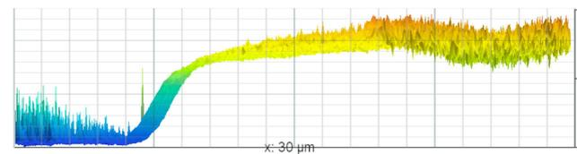
Figure 6: Shows a side view of a 3D reconstruction of a typical section of the edge of a TiN film using AFM. There is considerable variation across this step which can be seen on the light micrograph in figure 7. This variation settles out very quickly however away from the edge of the film.
