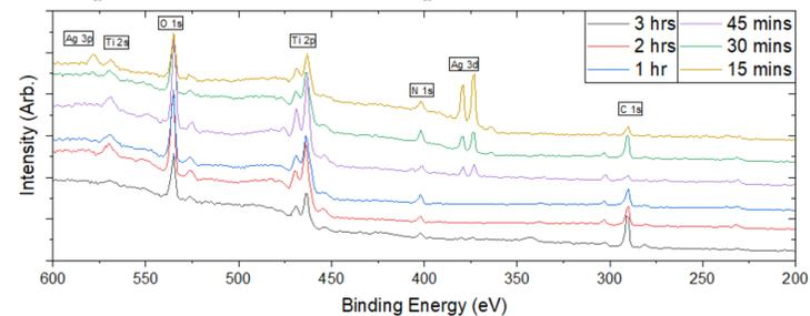
Figure 5: XPS survey spectra for the samples shown in figure 4. The intensity of the Ag 3d structure clearly indicates the increasing thickness of the TiN overlayer. The spectra are normalised and offset for clarity of presentation.
