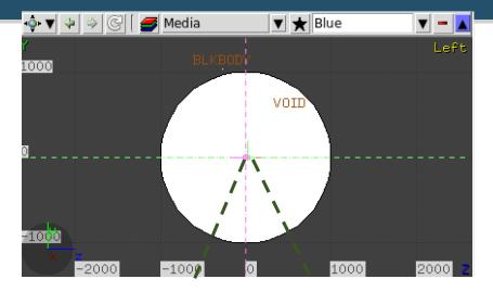
The whole geometry must be surrounded by a region of "blackhole" limited by a closed body.
