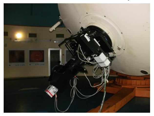
Observations with the focal reducer and in direct RC focus are carried out with ANDOR iKon-L BEX2-DD and ANDOR iKon-L E2V 42-40 CCD cameras (2048×2048 pixels,  $13.5 \times 13.5 \mu m$  size).
