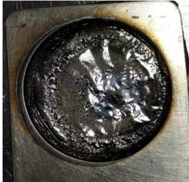
Target post-irradiation with I \sim 5 \mu\text{A}
