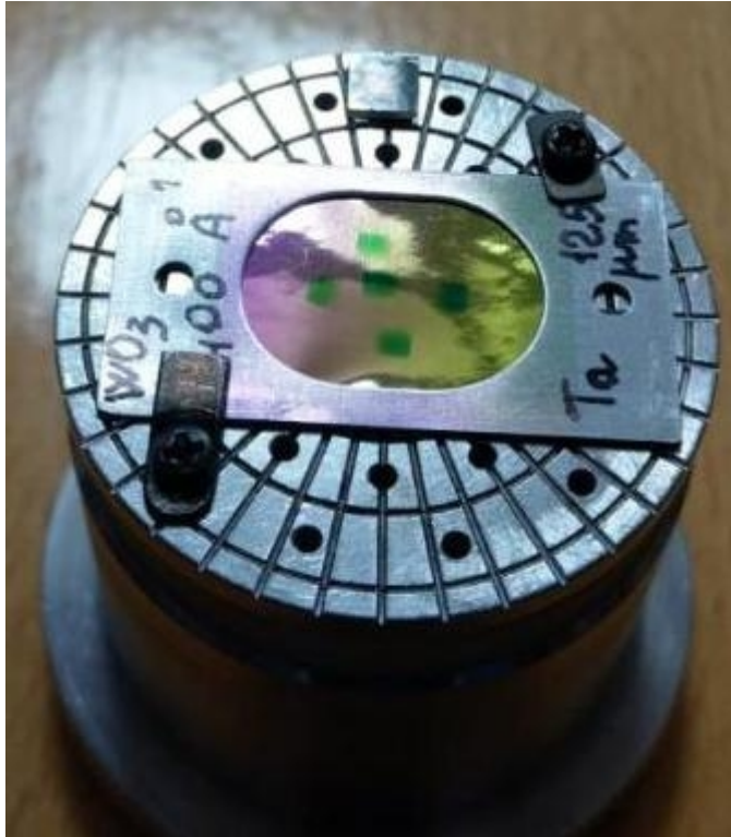
Target after RBS measurements
