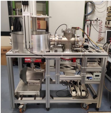
Target characterization: Alpha Particle Transmission spectroscopy @INFN-LNS
